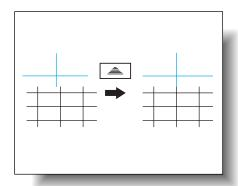
10 If the lines are shifted as shown at the right, touch [Y], and then touch to specify the desired negative adjustment for "Y" (between -1 dot and -6 dots).
